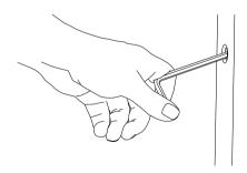
**4.** Tighten the frame adjusters clockwise, with a 5mm ball-ended Allen key, until the ends of the spreader plates are flat against the wall.
